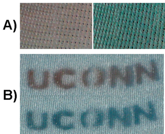
FIGURE 5. Images of (A) stretched, spandex fabric electrode in electrolyte bath switching an EC polymer from its neutral (left) to oxidized (right) states. (B) Stencil-patterned solid-state fabric ECD in its neutral (top) and oxidized (bottom) state.
